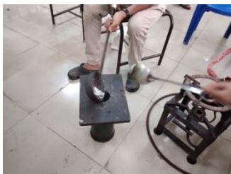
Fig. 3: Pouring melted yashada in Pitara yantra with oil
